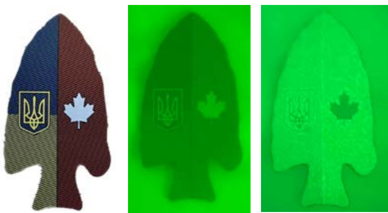
French made infrared patch introduced by Rotation 15 for usage in England. Night vision without IR filter (middle) and with IR illumination (right).
